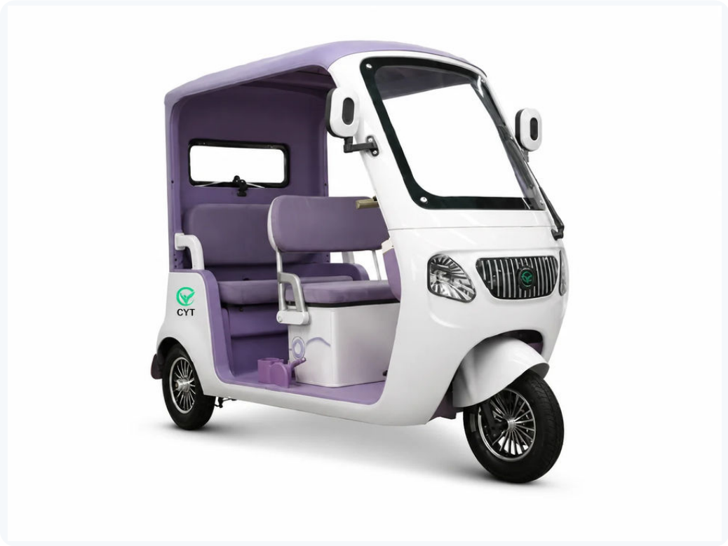
Electric passenger tricycle for short-distance travel.
