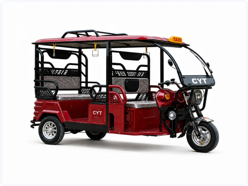
Electric passenger tricycle for short-distance travel.
